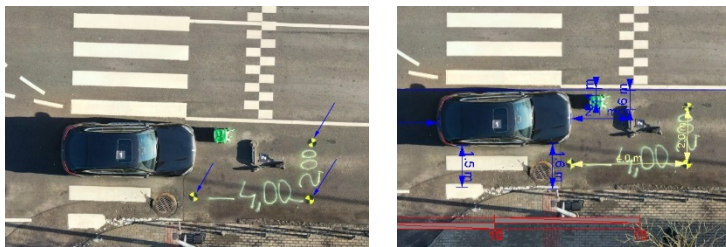
Fig. 1. Shows a photo of the terrain taken by a quadcopter with reference points, indicated by blue arrows on the left of the photograph, and the measured distances between the points, indicated on the right of the photograph
