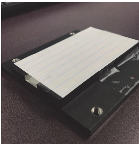
Fig. 10. Paper stretched tight and taped to flat metal mount
